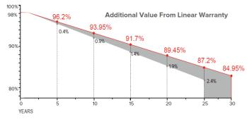
For PERC Monocrystalline Modules, the maximum loss of power output from the Peak Power at STC at the end of each year of the Power Warranty Period shall not be greater than (i) 2.0% plus (ii) 0.45%
