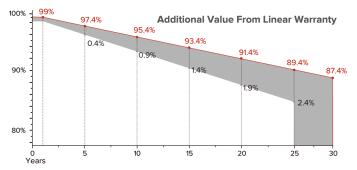
For N-Type Monocrystalline Modules, the maximum loss of power output from the Peak Power at STC at the end of each year of the Power Warranty Period shall not be greater than (i) 1.0% plus (ii) 0.4% multiplied by the number of years after the end of the first year of the Power Warranty Period (ending with no less than 87.4% at the end of the Power Warranty Period).
