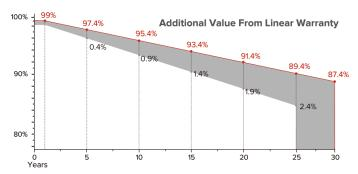
For N-type Monocrystalline Modules, the maximum loss of power output from the Peak Power at STC at the end of each year of the Power Warranty Period shall not be greater than (i) 1.0% plus (ii) 0.4% multiplied by the number of years after the end of the first year of the Power Warranty Period (ending with no less than 87.4% at the end of the Power Warranty Period).
