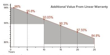
For PERC Monocrystalline Modules, the maximum loss of power output from the Peak Power at STC at
